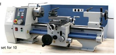
A reversible 2-mm pitch lead screw provides extended threading capability. You can create every American Standard Unified class 2A inch screw thread from 4 to 80 threads per inch, and you can create every American Standard Metric class 6h thread from 0.2 to 8 mm pitch with the change gears that are included.
